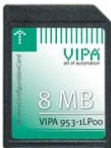
In front of the CPU there is a slot for storage media. For this, a MCC memory extension card is available from VIPA. The MCC is a specially prepared MMC (Multimedia Card). By plugging the MCC into the MCC slot and then an overall reset the according memory expansion is released. There may only one memory expansion be activated at one time. On the MCC there is the file memory.key. This file may not be altered or deleted. You may use the MCC also as "normal" MMC for storing your project.
