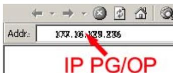
There is a web server, which can be accessed via the IP address of the Ethernet PG/OP channel with an Internet browser. At the web page information about the CPU and its connected modules can be found. ↪ [Chapter 5.6 'Hardware configuration - Ethernet PG/OP channel' on page 43](#)
